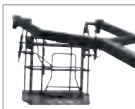
Pendular platform allows work under-bridges
