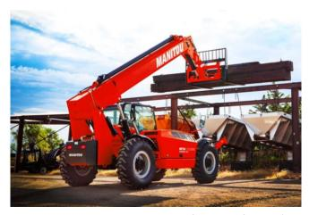
such as infrastructure, bridge and construction projects. With a turning radius of only 12 ft 2 in. (3.7 m), this model maneuvers on very tight work sites. Equipped with a 120 hp engine and powershift transmission, the MTA 12055 telehandler has a maximum travel speed of 22.8 mph. There is also easy access to the engine components to ensure ease of maintenance.
