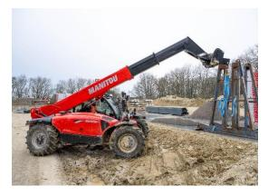
**6'6")**, have a broad selection of equipment. In the cab, the intuitive Harmony screen, with a display available in 22 languages, gives the operator real-time maintenance and usage notifications. This easy-to-use universal dashboard makes it quick to get to grips with and ensures the safety of both the operator and the machine. A new boom with built-in cylinder offers greater visibility for enhanced safety during loading and unloading. With their small size, these three models are **easy**
