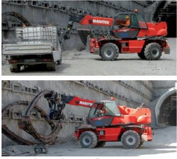
MRT 2150, the versatility per excellence: simultaneously aerial work platform, telescopic truck and crane!
