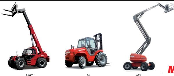
MHT Lifting: 8 - 10 m Capacity:6-22.5T M Lifting:3.7-4.8m Capacity: 3 - 7 T ATJ Workingheight:16-20m Maxoutreach:8.3-12m Numberofoperators:2
