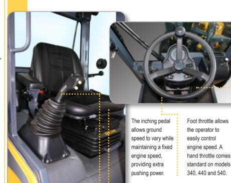
Multi-function joystick controls lift arm, bucket and float functions, as well as travel direction and auxiliary hydraulics. On models 340, 440 and 540, it controls two-speed and differential lock.
