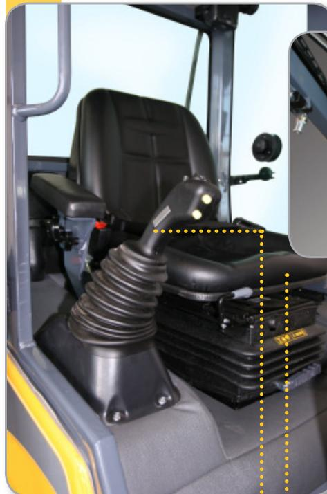
Multi-function joystick controls lift arm, bucket and float functions, as well as travel direction and auxiliary hydraulics. On models 340, 440 and 540, it controls two-speed and differential lock.
