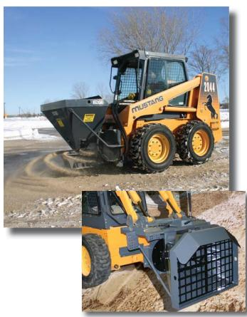
Self-feeding hopper with cutting edge
