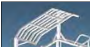
FOPS roof for a maximum protection
