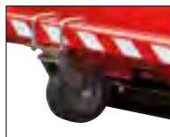
Swivel wheels for an easy driving process
